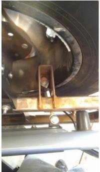
The tire carrier and tailgate open together in a single motion. Using the supplied tailgate plate and existing hardware, mount the plate with the 2 extension tabs to the top left-hand corner. These tabs will secure the heim assembly to the tailgate. The opposite side is bolted in to the extension bracket on the tire carrier itself.
