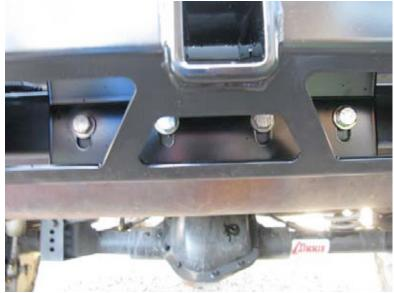
Using the supplied 9/16" x 4.5" bolts, mount rear section of bumper to the previously drilled portion of the rear support. Flat washers are used on the outside as shown. The lock washers are used on the inside. Hand tighten bolts at this time.
