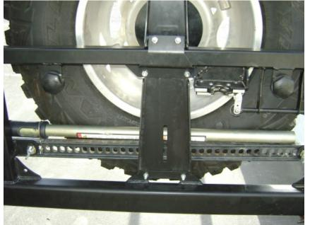
Install the supplied antenna/wheel post and corresponding backing plate as shown in the photo. The 5/16" carriage bolts will be used during this portion of the install. Also install the supplied urethane bumpstop with the corresponding 3/8" flat washer, lock washer and nut as shown in the photo. The backing plate and bump stops will be on the same side
