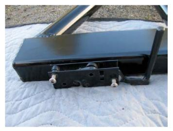
The latch mounts to the bottom side of the swing arm with the supplied 1/4" x 1.25" button head bolts. The arm extension should point in the same direction as the wheel mount (to the rear).
