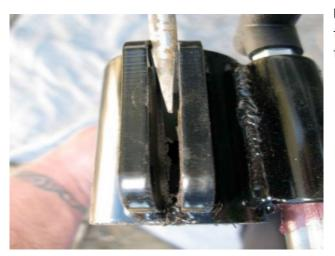
Using a large screwdriver or wedge, spread the pivot clamp to allow for installation on to the spindle bumper.
